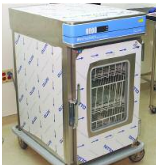
Figure 8. Fluid warming cabinet (EC770L, Entermics Medical System, Menomonee Falls, WI). The cabinet is warmed to 42°C using a low-heat-density electrothermal cable array to provide even heating of injection fluids. Solution warm-up time varies depending on cabinet warmer load. The cabinet cannot be used to warm blood.
