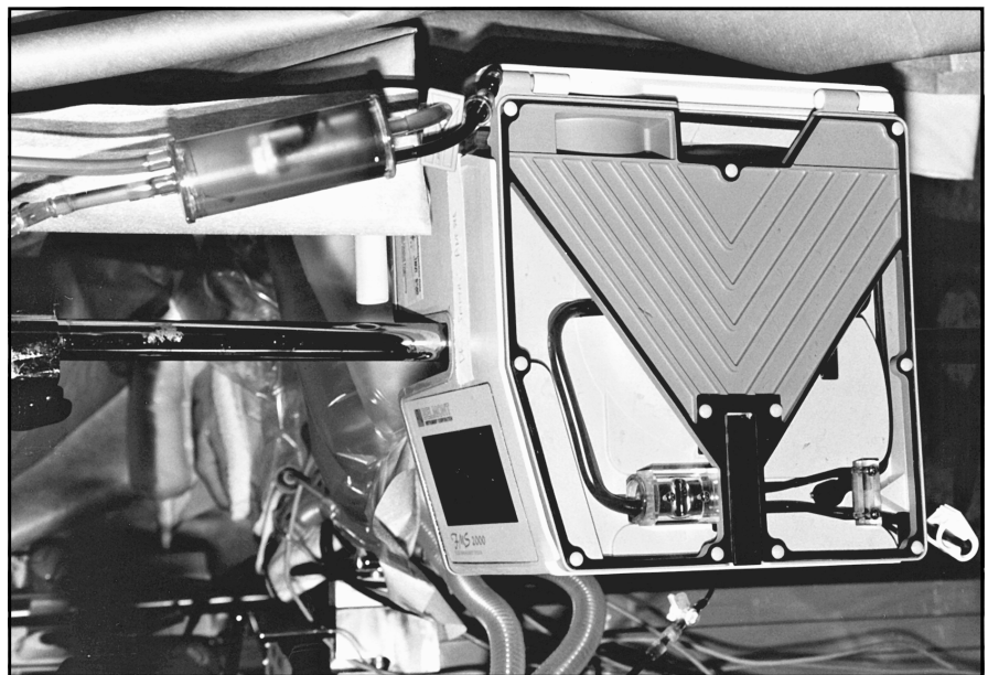
Figure 1. Belmont FMS 2000 warming system. The system consists of an integrated volumetric infusion pump coupled with a high-capacity magnetic induction heater. There are two ultrasonic air detectors—one at the fluid inlet and the other at the outflow to the patient coupled to an automatic shutoff.
